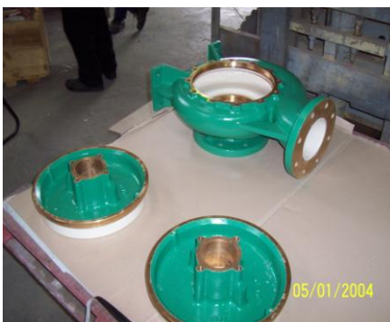
After external coating application
