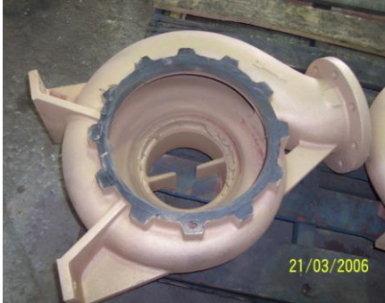
After masking and abrasive blasting
