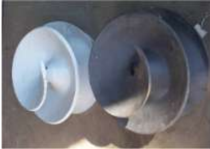
Refurbished on the left and new uncoated Impeller on the right
